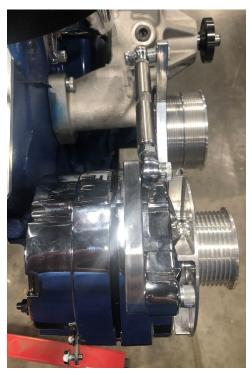
**Note**: This bracket is intended for both serpentine and V-belt applications. We recommend using Gates 8 Rib belts for serpentine and Gates Series 15 (13/32" Top Width) V-Belts.
