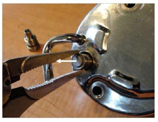
Step 1: Remove pressure union by unscrewing it counter-clockwise.
